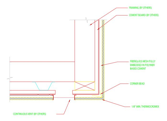
NOTE: All joints of cement board must be treated with 4" fiberglass mesh embedded in polymer based cement.
